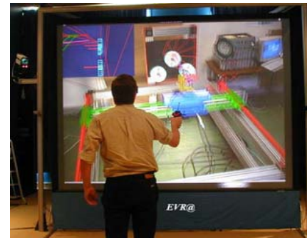
Mixed reality environment used for natural téléopération of a remote robot (LSC Mixed Reality Environment)
